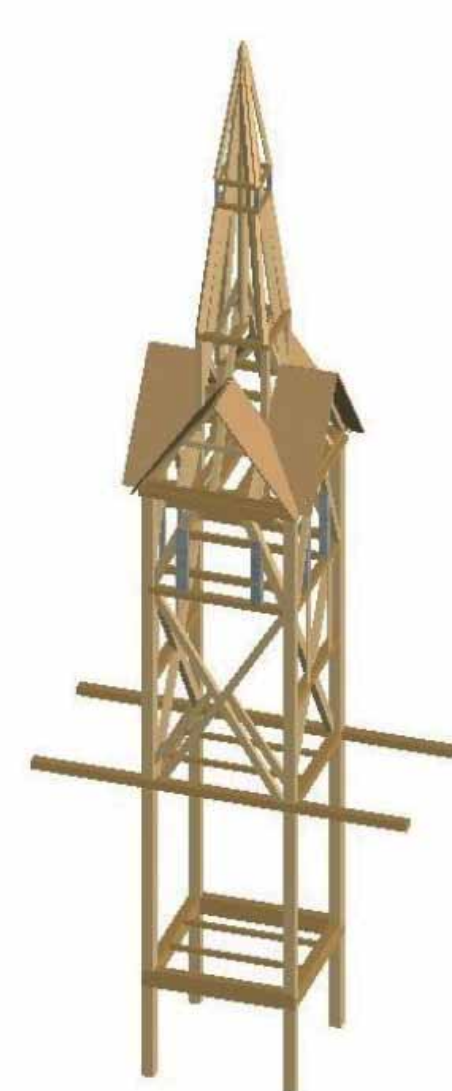
Fig.4. Axonometrics view of steeple timber structures
