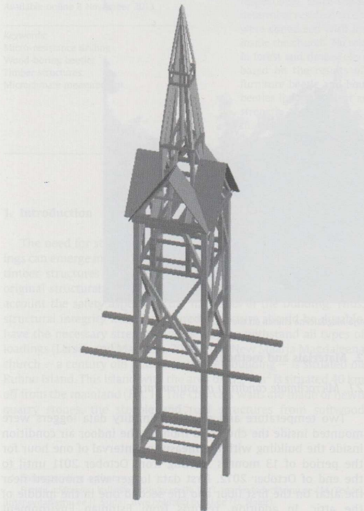
Fig. 3. Axonometric view of steeple timber structures of the New Maarja Magdaleena church.
