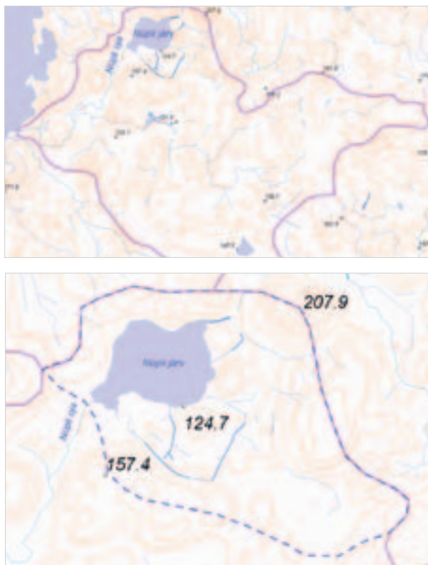
Figure 5.1.6. Catchment area of the Nüpli stream (pink contours), and on the scheme below, catchment area of Lake Nüpli, drawn on the basis of height contour lines (purple dashed line).
