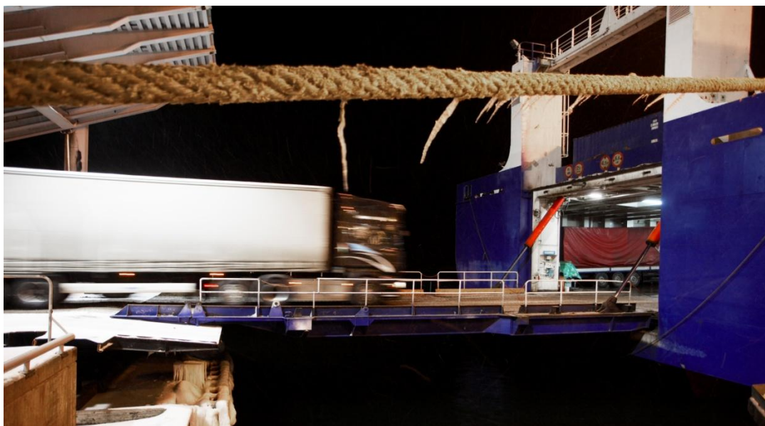
Figure 2: Ramps are a significant noise source in the vessel-quay interface. Photo: Per-Erik Adamsson/Ports of Stockholm.
