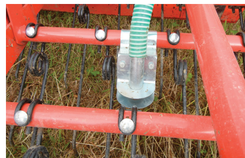
Seeds are blown out of the pipe on a long finger harrow.
