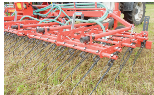
Detail of a long finger harrow.
