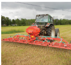
A long finger harrow sowing seed into a growing grass ley.
